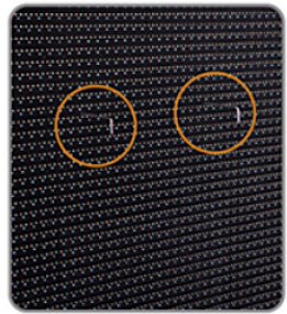
Insert tool into the maintenance hole
