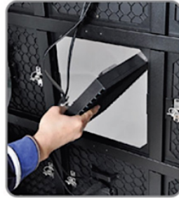
Take the module from rear directly
