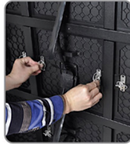
Manual unlock the module
