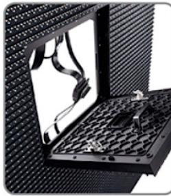
Disassemble cables, and take the module directly.
