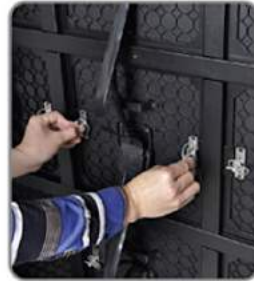
Manual unlock the module
