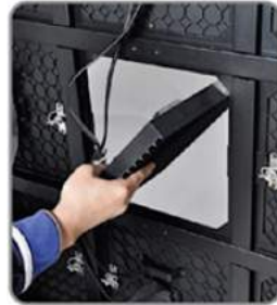
Take the module from rear directly
