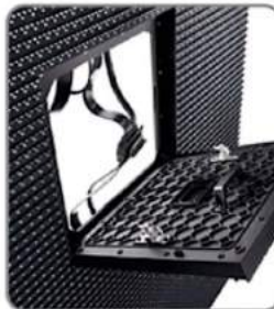
Disassemble cables, and take the module directly.
