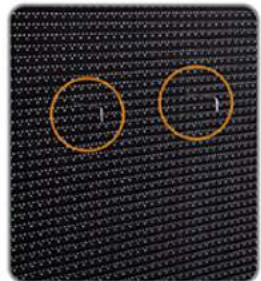
Insert tool into the maintenance hole
